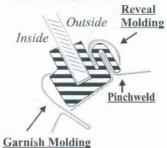
Lubricate the ¼" glass groove with glass lubricant or very soapy water to allow the glass to center itself while installing. Place new rubber on glass making sure that it is placed correctly and fits well. Any problems with fit will show up at this time. Rubber should fit glass without being too loose or too tight. Improper size will pucker or fold in corners.
